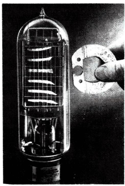
current or direct current power may be used to heat the filament and to supply voltages for the grid and plate. A tube socket and the adjustable voltage sources are all that are needed to permit the operation of the tube, although some meters will be of convenience in making adjustments and readings.
