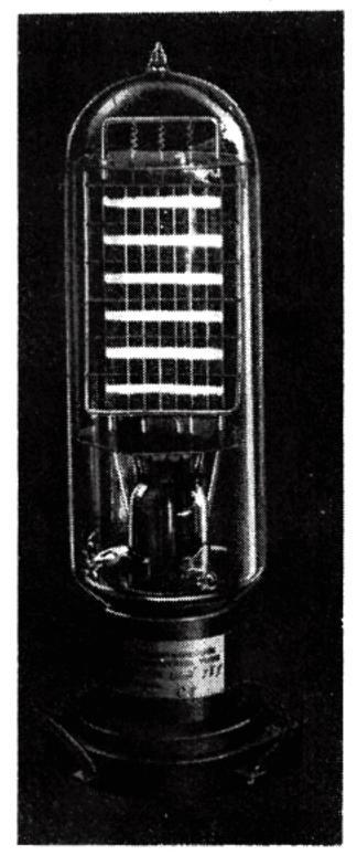
which condition there will be no electrons reaching the plate. The grid may be made still more negative, in which case there will be no apparent change in the tube, which voltage value corresponds with the conditions existing in an actual triode when the net voltage on the grid is greater than that required to produce plate current cutoff.
